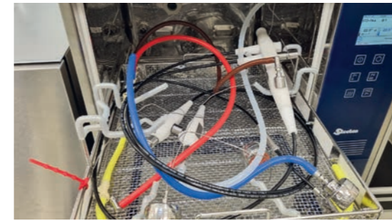
Figure 3: Spypach „Classic“ endoscope dummy with EB112 data logger for measuring pressures and temperatures in the simulated endoscope. Spypach „經典“內視鏡模型配有 EB112 數據記錄器，用於測量模擬內視鏡中的壓力和溫度。
