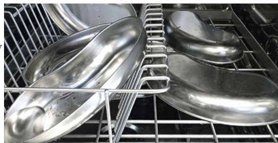
Fig圖. 3 Incorrect loading/kidney dishes that have toppled over. 不正確的裝載/腎臟盤倒塌了。
